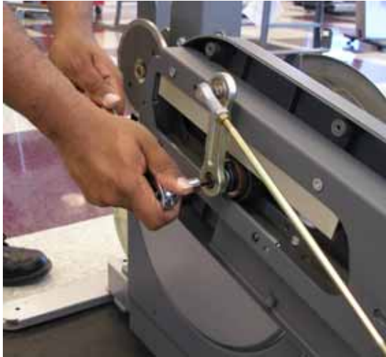
Fig. 5: removing the crank extension bolt
