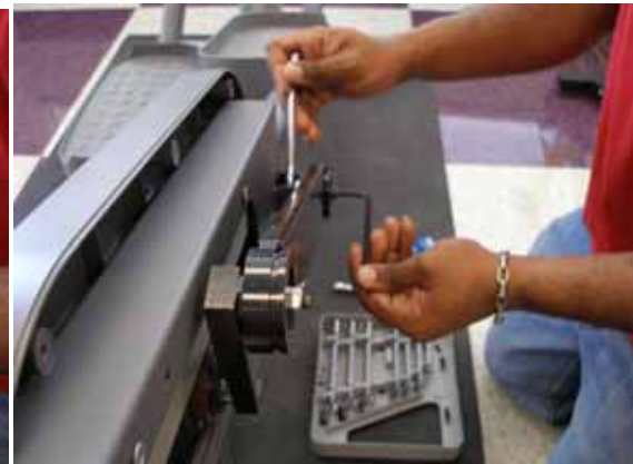
Fig. 8: installing the new control link assembly
